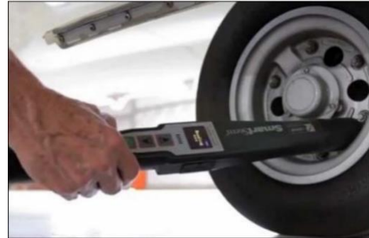
Figure 3. Reading data from a manometer [4]
